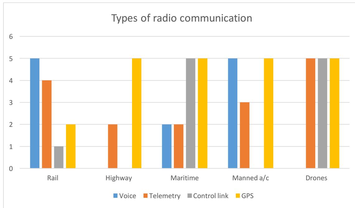
The importance of voice and control-link radio communication varies inversely with the presence of an onboard operator. If the vehicle is entirely remote-controlled, the control link is of great importance, and voice communication is irrelevant because there is no one with which to communicate on the vehicle.
